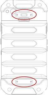
Align the hand strap assembly part with the screw hole on the top & bottom of the device's rear side.
